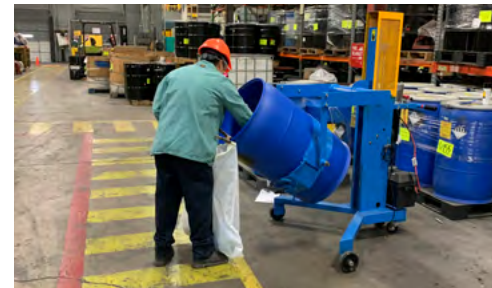
After assessment: Engineering solution facilitating access to the barrel contents for employees
