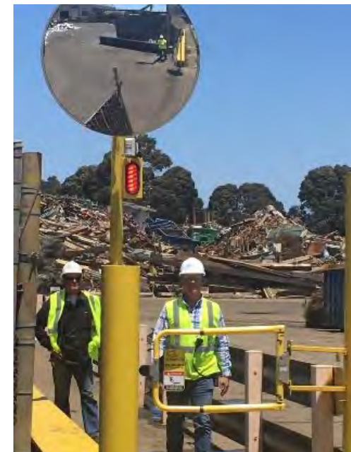
Using automated gates and blind spot mirrors to improve pedestrian segregation and visibility respectively
