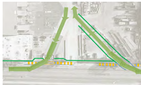
After: Traffic improvement, facilitating safe entry and exit to site without crossing into opposite traffic lanes
